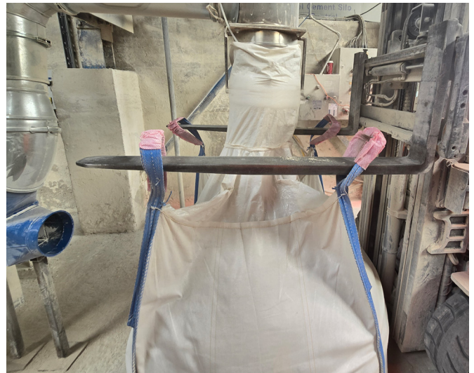
BFM® Bulk Bag Loader inflated during filling on site
