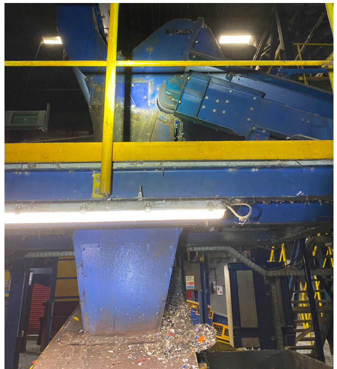
Daily cleaning on-and-around head drum on single conveyor
