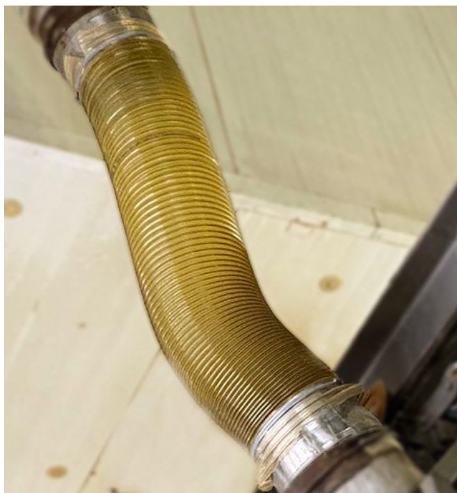
1.5m corrugated hose installed between the extruder & dryer
